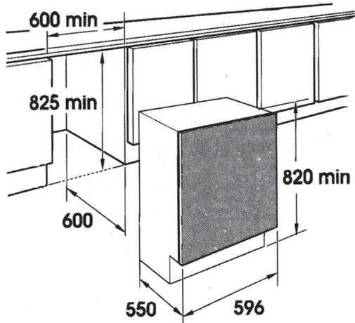
The four adjustable feet allow the height of the washing machine to be adjusted from 820 mm (by removing the nuts supplied and substituting with 5 mm nuts) to a max. 840 mm by raising the feet and blocking the lock nut to the base of the plate.
