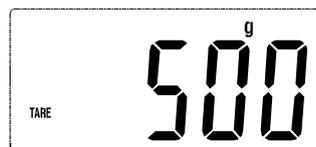
**Note:** If there is any operation the backlight will be off after about 10s and the scale will turn off automatically after about another 50s.
